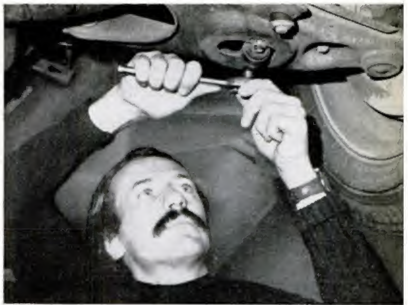
FRONT SHOCK is secured at its bottom end to the bottom A-arm. Two screws hold the shock's cross pin
